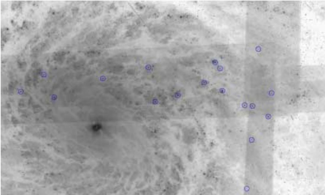
(c) Closeup showing stars used to measure intertile shifts and rotations, to register adjacent tiles in the mosaic
