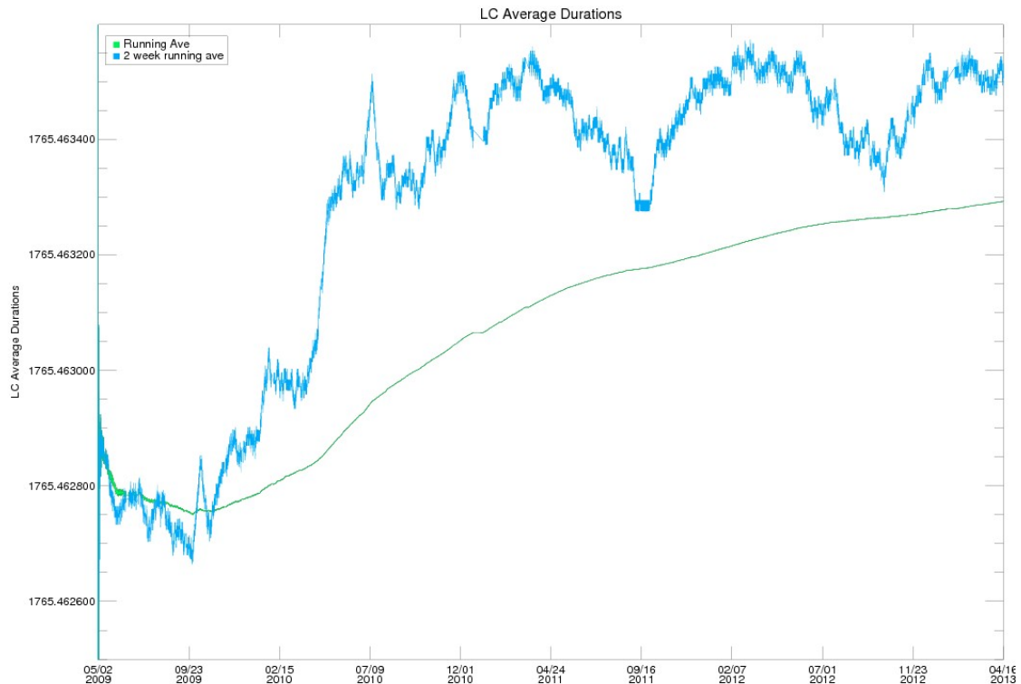
Figure 20: The change in the LC duration, given in seconds, with time, due to the drift in the onboard spacecraft clock. The two-week running average is plotted in blue, and the cumulative average with time is plotted in green. Each point on the green line is the median of all blue points from earlier epochs. The overall change is at the sub- millisecond level and therefore should not be of concern to the user.
