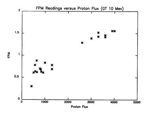
Figure 1. Correlation of FPM readings (volts) with proton flux (particles/cm/cm/ster/sec) for protons with energies in excess of 10 Mev.
