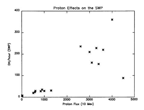
Figure 2. "Fogging" of the SWP camera, in DN/hour, due to protons. The proton flux, for protons with energies in excess of 10 Mev, is in units of particles/cm/cm/ster/sec. The proton flux and fogging rate are fairly well correlated, but there is a large scatter apparently due to variable amounts of shielding depending on the orientation of the spacecraft with respect to the incoming proton storm. The data are from the October sequence of proton storms.
