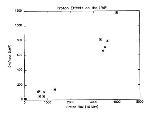
Figure 3. "Fogging" of the LWP camera, in DN/hour, due to protons. The units are the same as in Figure 2. Note that the LWP is 3 times as sensitive as the SWP to protons.
