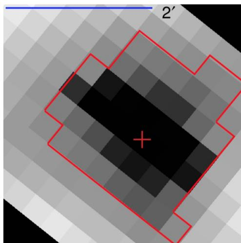
*Sample TESS target pixel file stack and aperture (TIC 261136679 shown here).*
