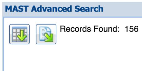
Figure 2: Buttons to load the Advanced Search results into the MAST Portal grid view (left) and download VO/CSV table of search results (right).
