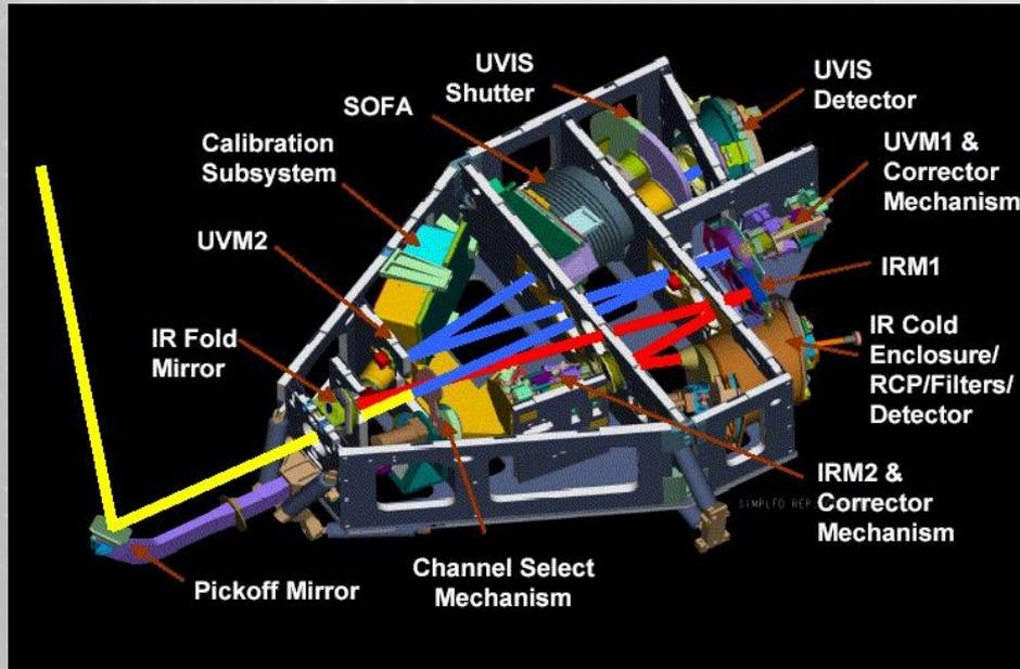
The WFC3 consists of two channels one operating in the optical/ultraviolet and one in the near-infrared.
