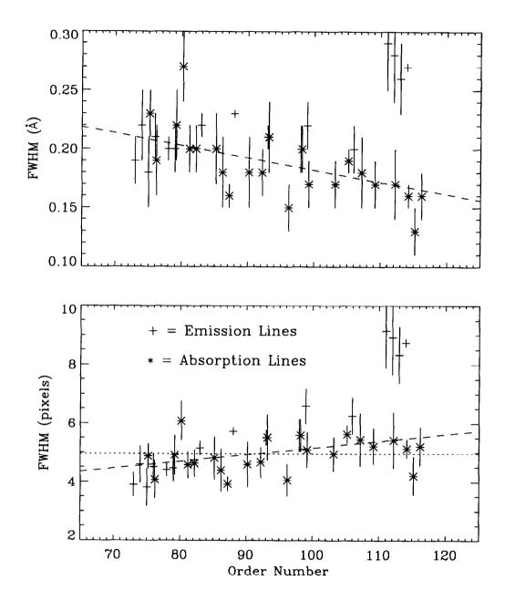
Figure 16: SWP high-dispersion spectral resolution from small-aperture stellar-source analysis. Emission line measurements for orders 111 and above were excluded from the fits. Emission line data is horizontally offset to the left of the absorption line data by half an order.
