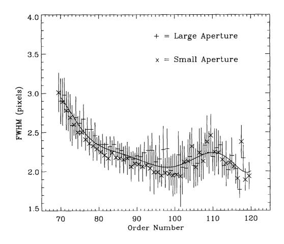
Figure 4: LWP high-dispersion spatial resolution for sample position 507. Small-aperture data is horizontally offset to the left of the large-aperture data by half an order.
