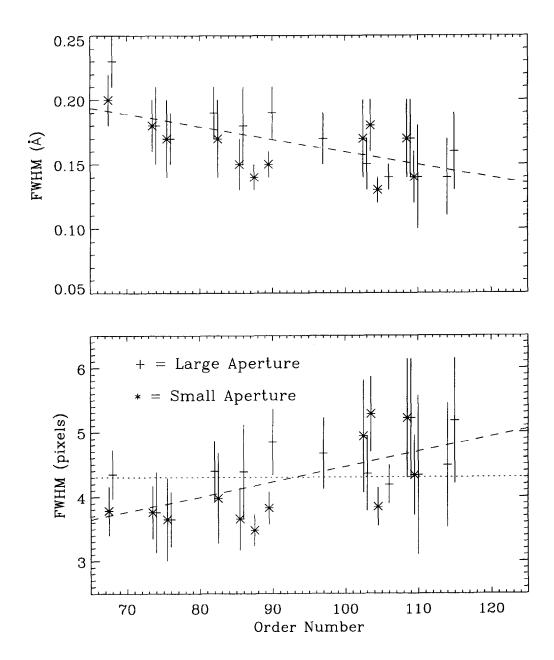
Figure 14: SWP high-dispersion spectral resolution from analysis of largeand small-aperture Zeta Oph data. Small-aperture data is horizontally offset to the left of the large-aperture data by half an order.
