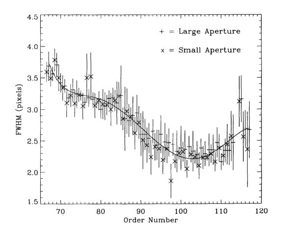
Figure 9: SWP high-dispersion spatial resolution for sample position 507. Small-aperture data is horizontally offset to the left of the large-aperture data by half an order.
