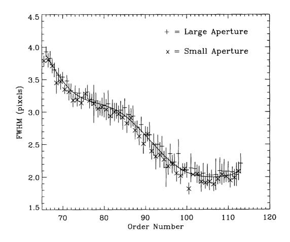
Figure 8: SWP high-dispersion spatial resolution for sample position 384. Small-aperture data is horizontally offset to the left of the large-aperture data by half an order.
