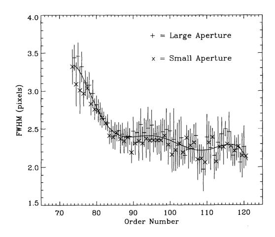
Figure 5: LWP high-dispersion spatial resolution for sample position 615. Small-aperture data is horizontally offset to the left of the large-aperture data by half an order.
