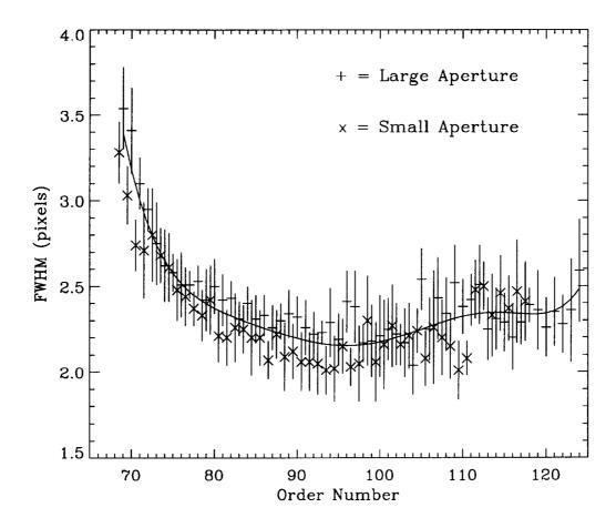
Figure 3: LWP high-dispersion spatial resolution for sample position 384. Small-aperture data is horizontally offset to the left of the large-aperture data by half an order.
