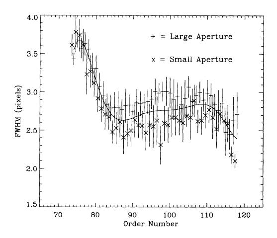
Figure 1: LWP high-dispersion spatial resolution for sample position 134. Small-aperture data is horizontally offset to the left of the large-aperture data by half an order.
