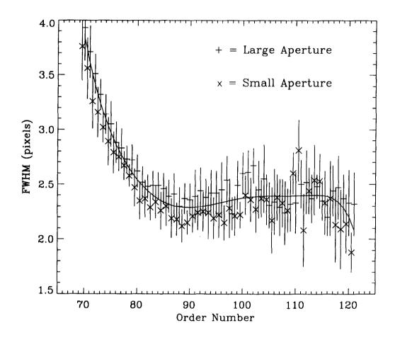
Figure 2: LWP high-dispersion spatial resolution for sample position 258. Small-aperture data is horizontally offset to the left of the large-aperture data by half an order.
