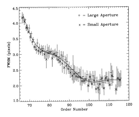
Figure 7: SWP high-dispersion spatial resolution for sample position 258. Small-aperture data is horizontally offset to the left of the large-aperture data by half an order.
