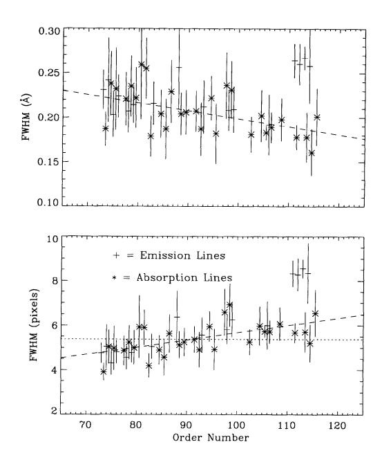
Figure 15: SWP high-dispersion spectral resolution from large-aperture stellar-source analysis. Emission line measurements for orders 111 and above were excluded from the fits. Emission line data is horizontally offset to the left of the absorption line data by half an order.
