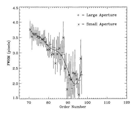
Figure 10: SWP high-dispersion spatial resolution for sample position 615. Small-aperture data is horizontally offset to the left of the large-aperture data by half an order.
