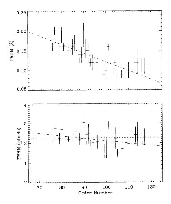
Figure 13: LWP high-dispersion spectral resolution from analysis of large-aperture Zeta Oph data.
