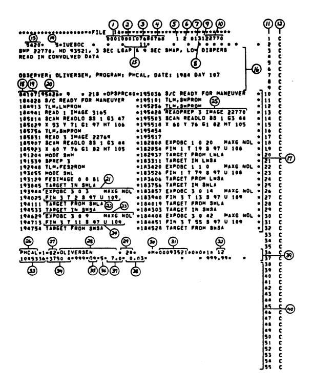
Figure 5a: Print of science image header for raw image (RI) file. (Reproduced from Turnrose and Thompson, 1984)
