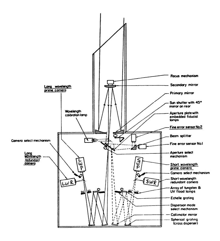
Figure 1: Optical schemetic of the IUE scientific instrument
