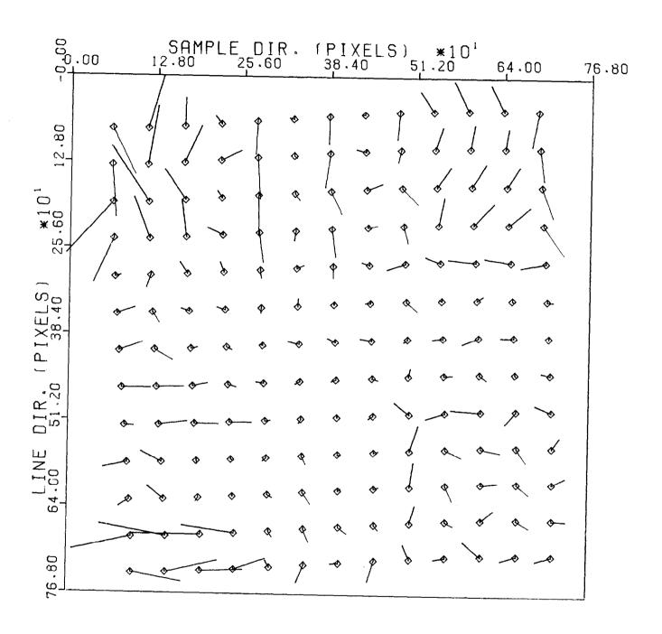
FIGURE 4 - Displacements of smoothed mean reseaux from mean reseaux, LWR (Magnified by 80)
