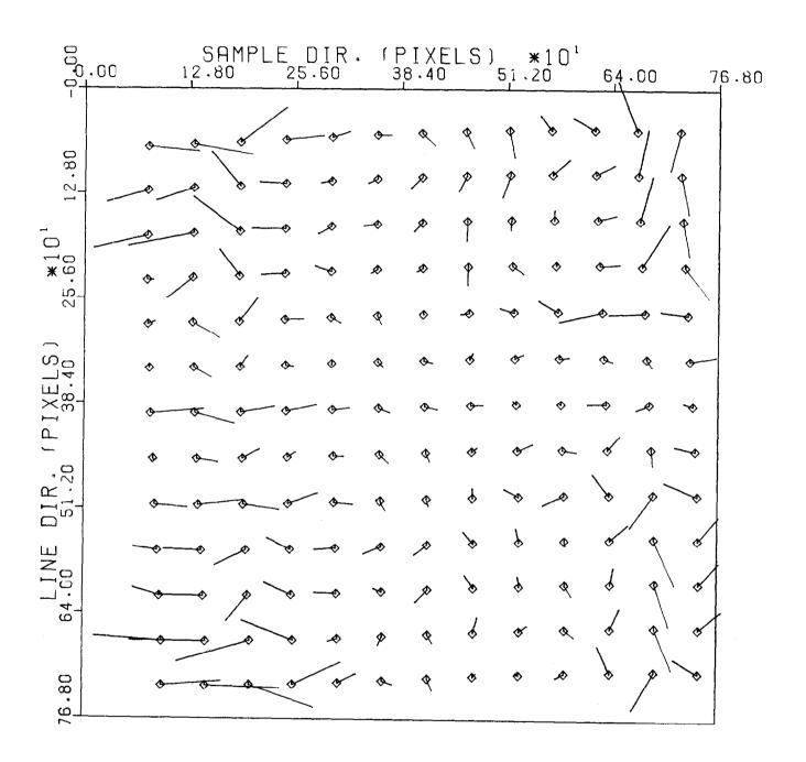
FIGURE 3 - Displacements of smoothed mean reseaux from mean reseaux, SWP (Magnified by 80)
