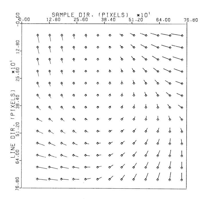
FIGURE 1 - Displacements of mean reseaux from correct grid, SWP (Magnified by 2)
