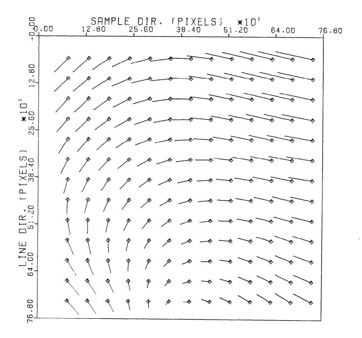
FIGURE 2 - Displacements of mean reseaux from correct grid, LWR (Magnified by 2)
