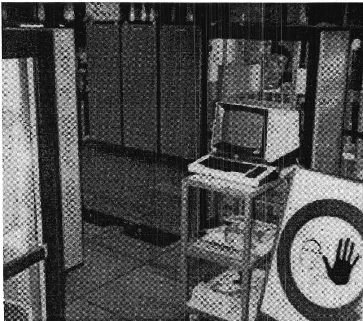
Picture: Dismantling of the IUE R/T computer 'Telefile-85' - December 1996 (Front right: rack still holding T-85 CPU; Back: backside of the racks holding the magtape drives)
